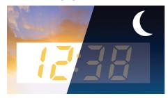
Always be assured of being able to read the display, whatever time of day it is. The built-in light sensor reads the intensity of ambient light and then determines how bright the display needs to be to ensure clarity. During the day, or under strong lighting, the brightness automatically increases so you can see the display easily against the surrounding flood of light. At night, or under very low light conditions, the display softens, allowing you to look at the display without discomfort, and
